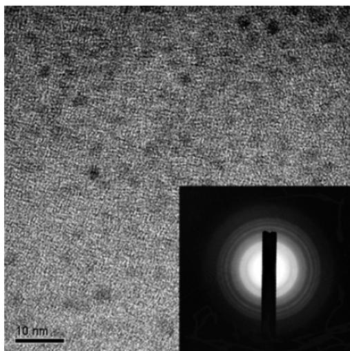
**Figure 1.** TEM image with the electron diffraction pattern in the inset for ZnO(PEGME350) nanocrystals prepared using the molar ratio  $[\text{LiOH}]/[\text{Zn}] = 1.4$ .
