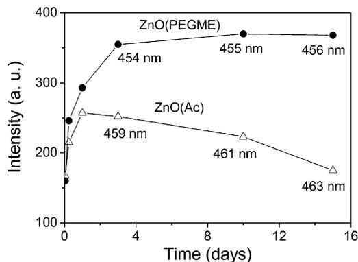
**Figure 3.** Emission peak intensity and position versus storage time for ZnO(PEGME350) and ZnO(Ac) ethanol colloid solutions prepared with the same molar ratio  $[\text{LiOH}]/[\text{Zn}] = 3.5$  and zinc concentration  $[\text{Zn}] = 0.01 \text{ M}$ .
